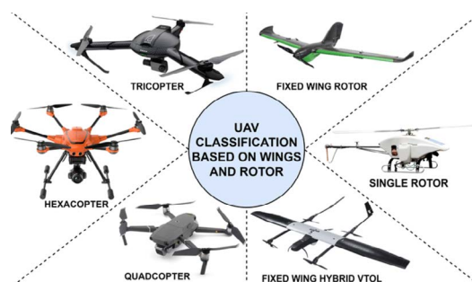
EXHIBIT 5 - CLASSIFICATION OF UAVS BASED ON WINGS AND ROTORS
